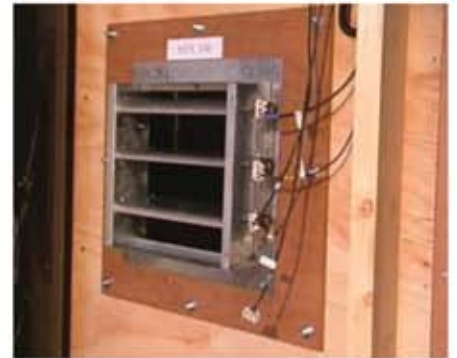
Blade positions at peak pressure of 251PA - as shown on SHX 300 GD2 data logging sheet.
